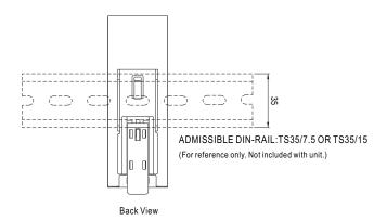
This series fits DIN-RAIL TS35/7.5 or TS35/15. For installation details, please refer to the USER MANUAL on http://www.meanwell.com/search/NDR-120/NDR\_manual.pdf
