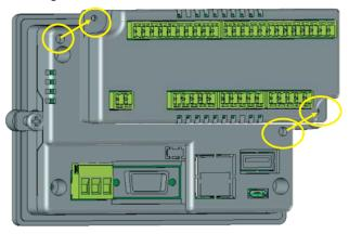
For 7" and 10.2" HMI models, the procedure of mounting expansions is same. Only instead of horizontal mounting, expansions will mount in vertical directions.
