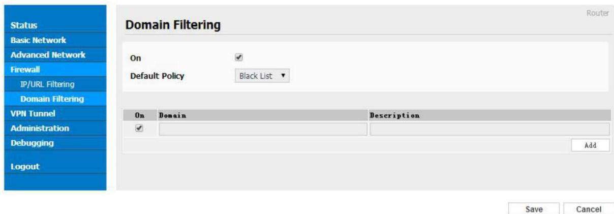
Figure 3-15 Domain Filtering Setting GUI
