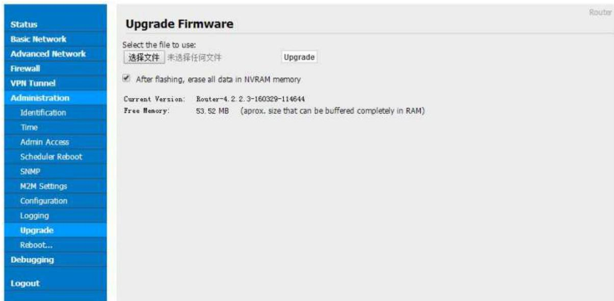
Figure 3-10 Firmware Upgrade GUI
