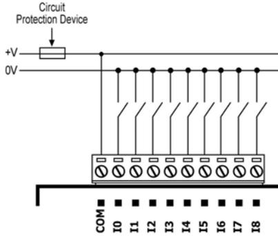
pnp (source) digital input wiring
