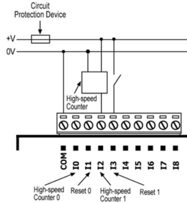
Inputs I0, I1, and I2, I3 can be used as shaft encoders as shown below.
