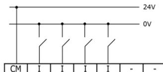
High Speed Input wiring, sink
